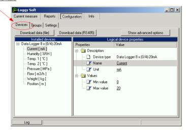
Fig. 3.12. **Configuration – Devices** tab (advanced options hidden)
