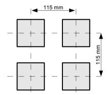
Fig. 4.4. Minimum distances when assembly of a number of units
