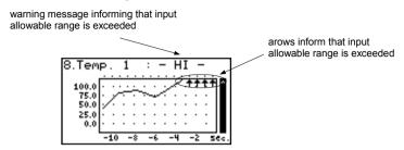
Fig. 6.15. Exceeding the upper limit of the allowable measurement range
