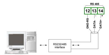
Fig. 4.10. Connection of RS-485 transmission signals
