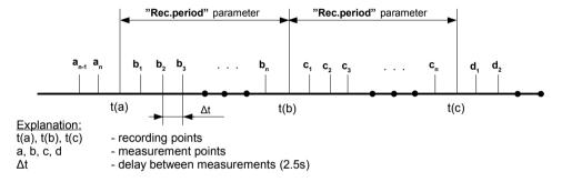
Fig. 6.2. Principle of measurement recording
