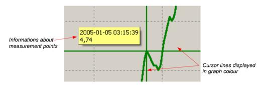
Fig. 3.9. Graph with special tracking cursor
