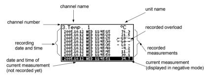
Fig. 6.11. Unit in "Measurements list" measurement results presentation mode. "List type" parameter set as "current".
