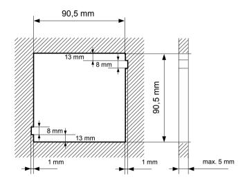
Fig. 4.1. Mounting hole dimensions
