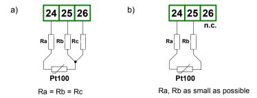
Fig. 4.9. Connection of Pt100 sensors for channel no 1: a) 3-wires circuit; b) 2-wires circuit;
