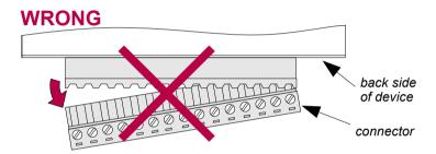
Fig. 4.3. Connectors removing method
