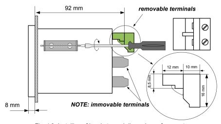
Fig. 4.2. Installing of brackets, and dimensions of connectors.
