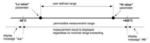
Fig. 6.1. Definition of measurement ranges
