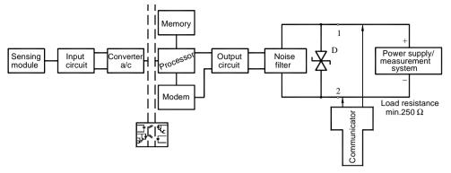
Fig.1. APT... transmitters - block diagram.
