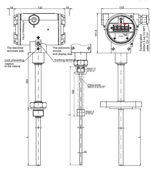
Fig.3. APT-2000ALW smart temperature transmitter
