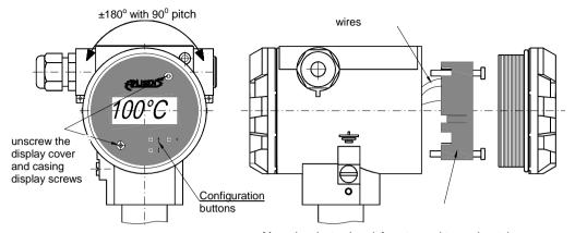
Move the electronic unit from transmitter casing, take up the upper part of the casing with display from the catch and revolve its to left or to right to the display setting at needed position.
