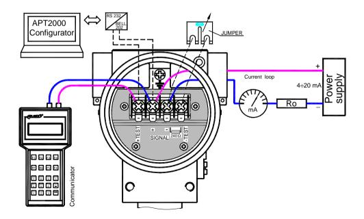
Fig.2c. The link of transmitter and communicator or modem to <SIGNAL+> <TEST+> transmitter terminals in case of the resistance in current loop is smaller than 250 $\Omega$ .
