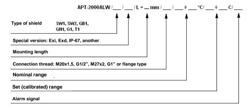
Example: Temperature transmitter APT-2000ALW, shield T1, version Exi, mounting length 250 mm, connection flange DN50 PN40, nominal range: -40 do 550 °C, calibrated range: 0 do 300 °C, alarm signal for example 23 mA.
