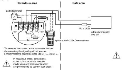
The transmitter is equipped in additional communication resistor RD = 240  $\Omega$ .
