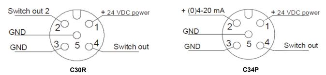
Micro-DC Cable Color Codes: Brown=Pin 1; White=Pin 2; Blue=Pin 3; Black=Pin 4; Gray=Pin 5
