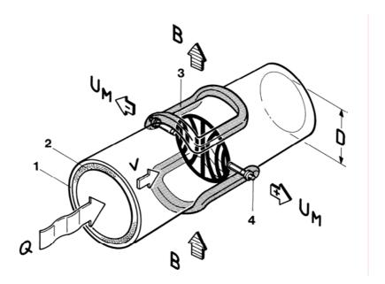
Through a meter tube provided with an insulating lining a liquid flows at velocity v and a flow rate Q, producing a measuring-circuit voltage Um at the two electrodes at right angles to the direction of flow. The size of this measuring-circuit voltage is proportional to the mean flow velocity and the volume flow rate.
