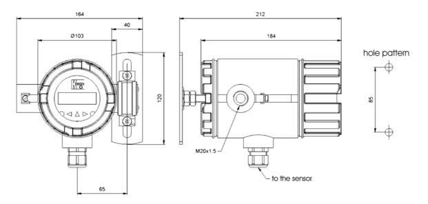
Transmitter type UMF2 with wall bracket
