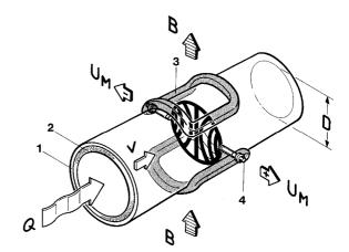
A fluid with a flow velocity v and a flow rate Q flowing through a tube (1) with an insulating lining (2)
