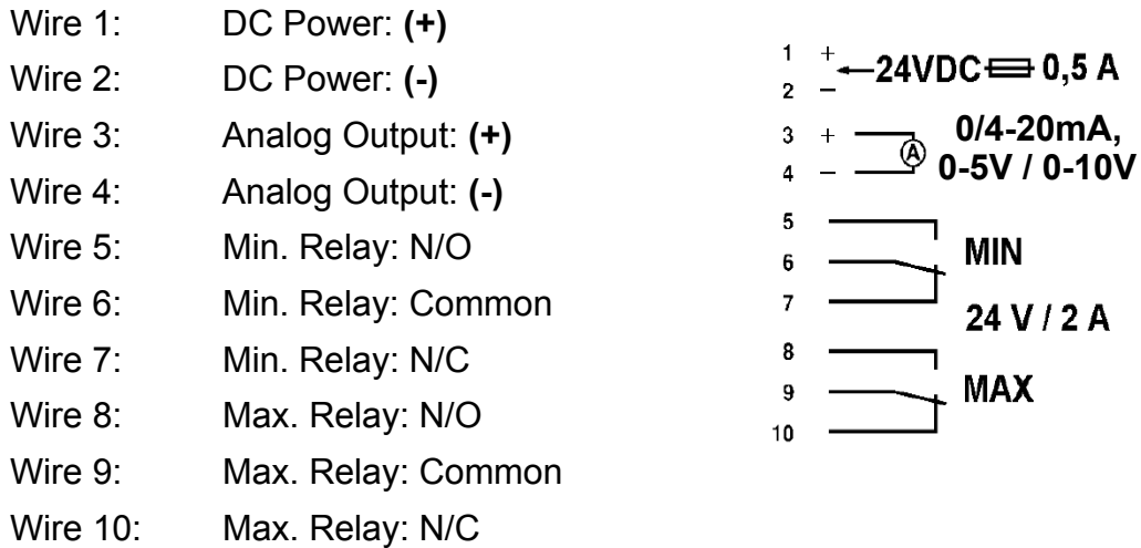
Diagram 3.2: Wiring for Optional Electronic Controller
