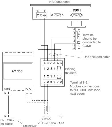
Note: NB 9000 COM1: Modbus D1 = Pin 1 and 4. Modbus D0 = Pin 8 and 9. Cache = shield.
